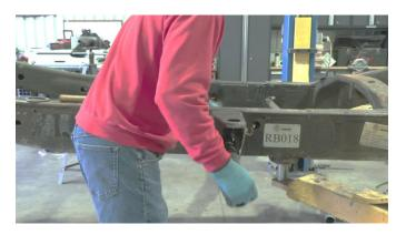
Slide the crossmember through to the opposite side of the frame rail. Then, position the two inner plates against the inside surfaces of the frame rails.
