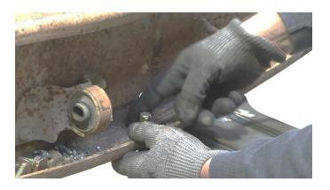
After screwing in your hardware, tighten them with a 14mm socket and 15mm wrench.
