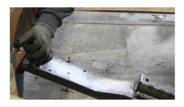
After screwing in your hardware, tighten them with a 19mm socket and 18mm wrench.
