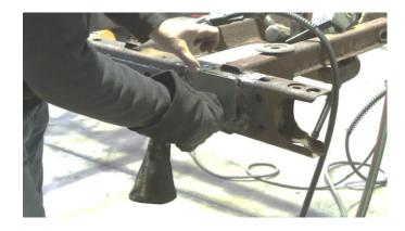
Following proper welding procedures, tac weld your frame plate onto the frame.
