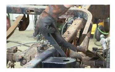
Grind the work area free of rust and debris, revealing bare metal/ followed by coating the work area with a weld through primer to help prevent against further rust development.
