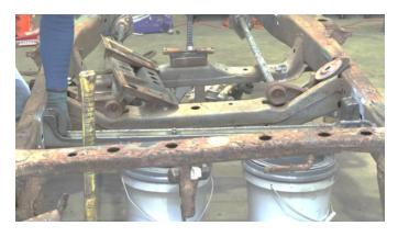
Following proper welding procedure, tac weld your crossmember into place before welding it on fully. Weld 100% around all edges.
