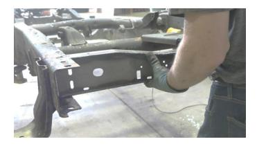
Then, following proper welding procedures, tac weld your crossmember into place before welding it on fully. Weld 100% around all edges.
