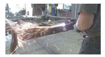
Then, cut out the rear frame crossmember and any obstructions in the work area. You can cut your crossmember in half to make it easier to remove.
