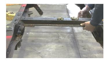
After your bolts are screwed into place, use a 14mm socket and 15mm wrench to tighten your hardware.
