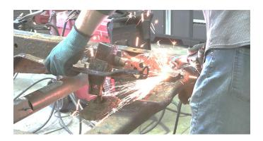
Grind the frame free of rust and debris, revealing bare metal. Be careful not to grind through your crossmembers.
