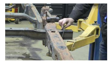
Following proper welding procedures, tac weld your crossmember and its plates to the frame before welding it on fully. Weld 100% of all edges.
