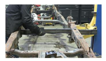
Once the crossmember is in place, use a tape measure to ensure both sides are of equal length. We measured approximately 5 % inches from the end of the crossmember to the outer side of the frame rail.
