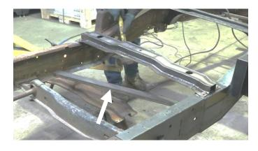
Then, take your two support brackets and hold them up to the underside of your frame, lining up the holes with your crossmember. Once you have the holes aligned, screw in the twelve remaining screws and nuts.
