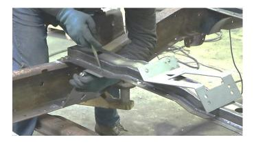
Once you have all of your hardware screwed into place, tighten your hardware with a 15mm socket and wrench.
